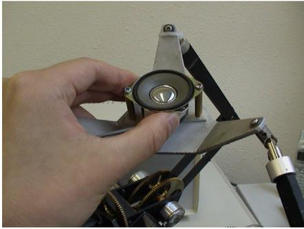
**Figure 2:** Speaker at the end effector of HapticMaster
