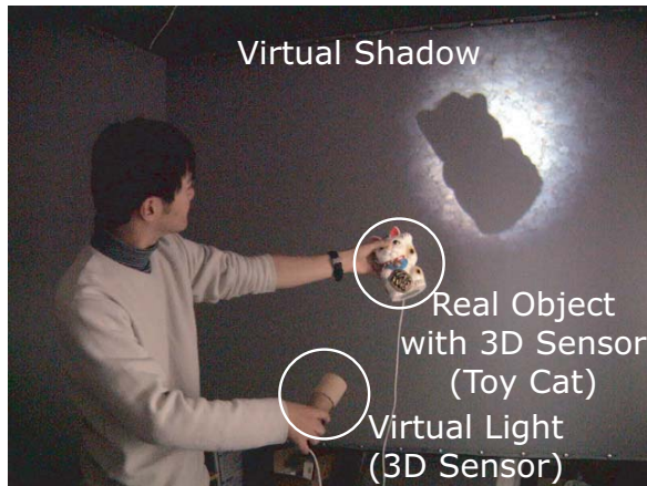
(a) RV Shadow for rigid objects (Sect.5.1): The shape of a real object (a toy cat) is measured in advance and utilized for displaying its shadow onto a virtual wall.
