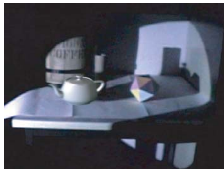
(d) A teapot is superimposed. We can see that the projected VR shadow matches the superimposed virtual object.
