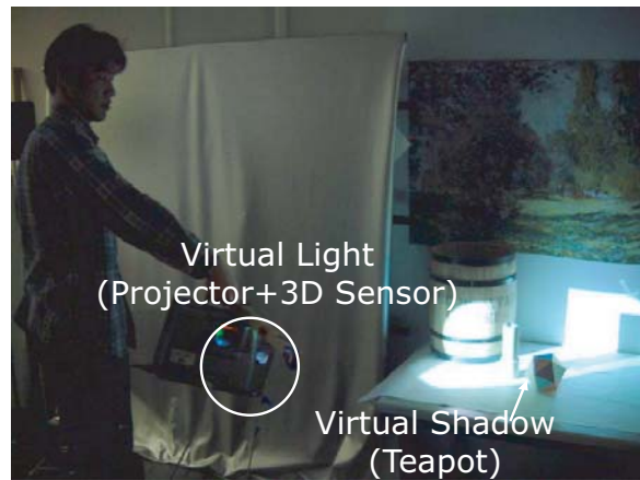
(d) VR Shadow (Sect.5.4): The shadow of a virtual object (a teapot) is projected onto the real world. We can see just the shadow, and we need an additional display (See-through HMD) to see the teapot itself.
